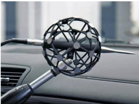
With the innovative Scan 3D probe, the sound can be “visualized” in the STS Acoustic Lab.
